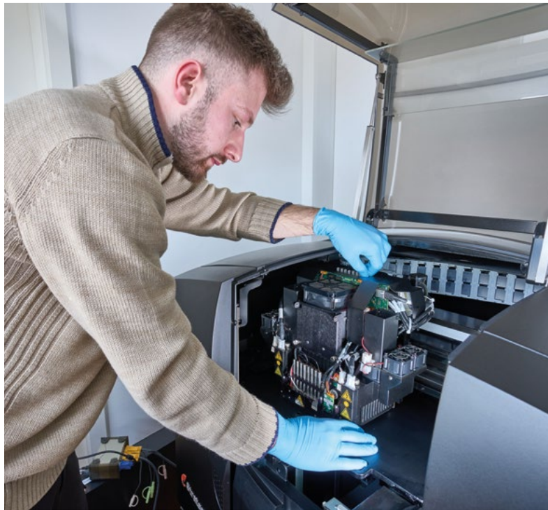
Adrian Jaeger checks and cleans the print heads before a 3D print
